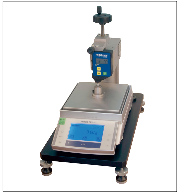
DUROMETER CALIBRATION DEVICE/FORCE
